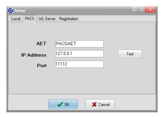
This is the remote PACS configuration: AET, IP Address and Port Number. The Test Button is for sending a DICOM Echo to the remote PACS.
