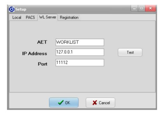
This is the remote Worklist configuration: AET, IP Address and Port Number. The Test Button is for sending a DICOM Echo to the remote Worklist.
