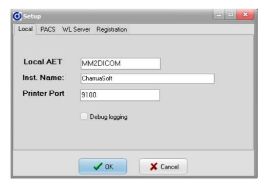
Local settings are configured here, DICOM AET, "Institution Name" for the DICOM convertion, and also the LPR port for the XPS2DICOM printer.
